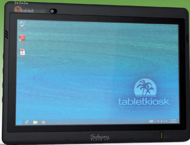
Sahara Slate PC® i575 Tablet PCs feature a 3rd Generation Intel® Core™ i7 vPro™ processor, up to 16GB RAM, user upgradeable SSD and optional dual mode digitizer+touch, LCD display with chemically strengthened glass and runs Windows® 7 and Windows® 8.
